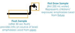
v. Sampling should proceed from "upstream to downstream" (i.e., from closer to where the water first enters the building to further away), which avoids inadvertent sampling-induced flushing of the lines
